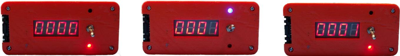
Figure 7: Using the FTE interface to set the test point number and active mode
