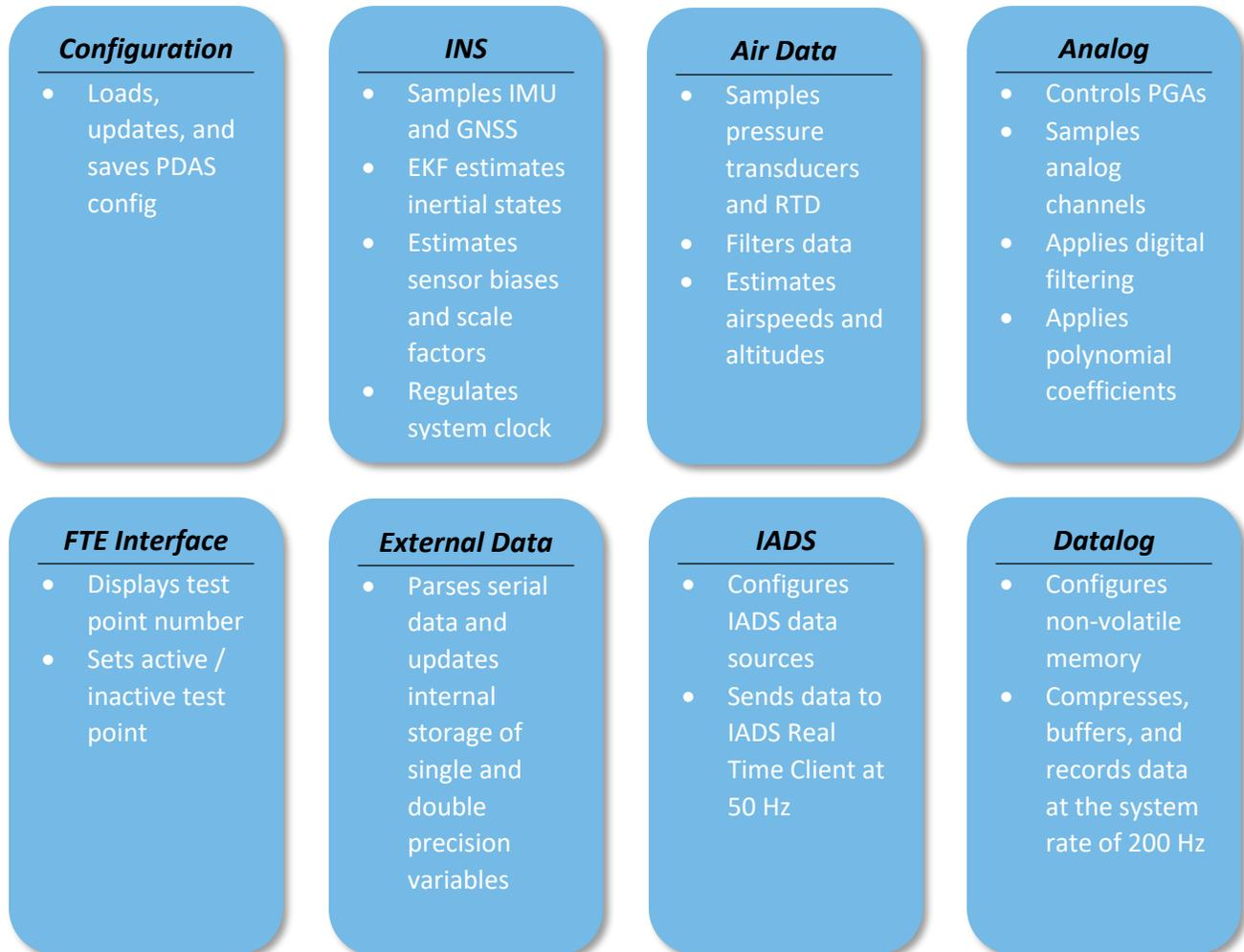
Figure 1: PDAS software modules.
