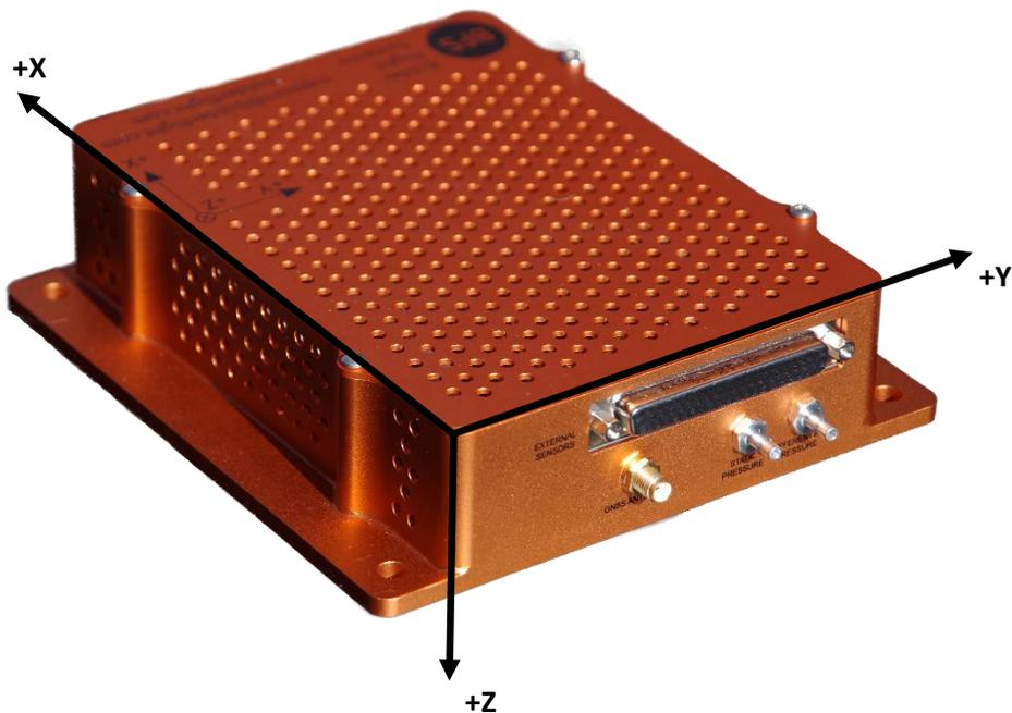
Figure 4: PDAS coordinate system
