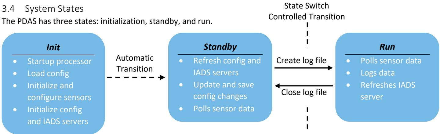
Upon receiving power, the PDAS automatically transitions through the initialization state and enters the standby state. In the standby state, all of the software modules are active except for datalog. In this state, you can view PDAS data via the web server or IADS server, modify the PDAS configuration, and download or delete data log files from the PDAS storage.
