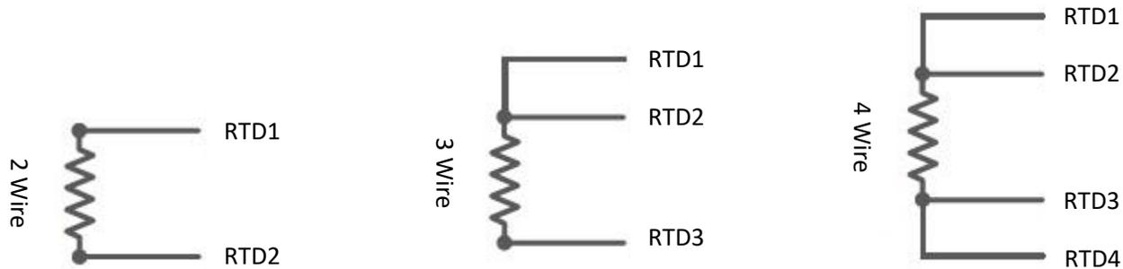
Figure 8: RTD wiring
