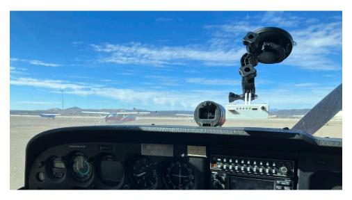
Figure 9: Example installation of OnFlight Hub aligned with aircraft reference frame.
