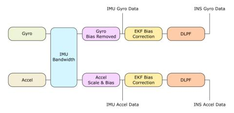
Figure 2: IMU data flow.
